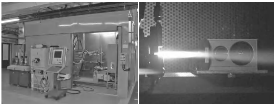
Figure 16.6. Atmospheric plasma-spraying unit (left) and plasma torch with particle diagnostic system (right).
