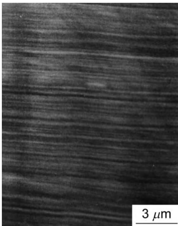
Figure 8.18. SEM micrograph of the polished cross section of an amorphous CVD \text{Si}_3\text{N}_4 -BN composite (50 mass % BN).
