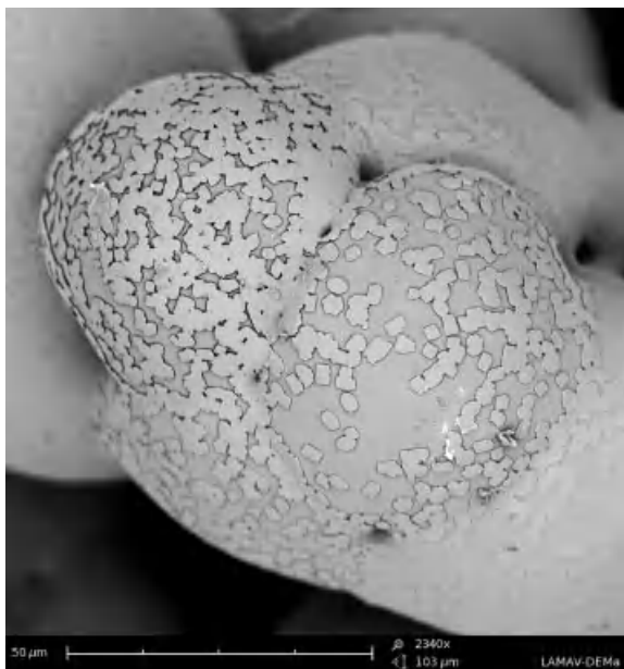
Figure 3.29. SEM micrograph of diopside surface crystals grown during sintering at 810°C for 120 min from diopside glass microspheres spherodized in gas flame [168].
