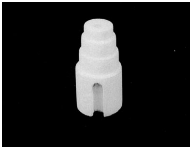
Figure 6.11. Photograph of machined Al 2 O 3 green body with a 6 wt % binder showing recessed steps by lathing, a center cavity by drilling, and a groove by milling. Reprinted from Reference 14 with permission from Elsevier.
