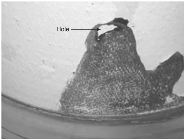
Figure 10.9. After about 14,000 h of field testing, the inner Hi Nicalon/SiC-Si liner made by melt infiltration shows a hole in the environmental barrier coating layer (reprinted from J. Kimmel, N. Miriyala, J. Price, K. More, P. Tororelli, H. Eaton, G. Linsey, and E. Sun (2002) Evaluation of CFCC liners with EBC after field testing in a gas turbine, Journal of the European Ceramic Society , 22[14–15] 2769–2775, with permission from Elsevier).
